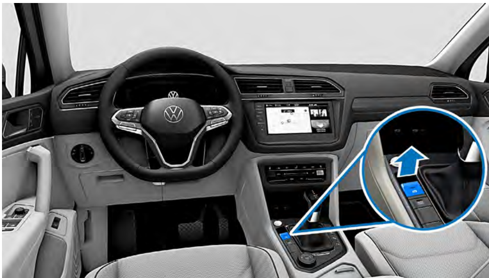
Conventional vehicle with automatic gearbox: apply electronic parking brake or pull handbrake lever.
