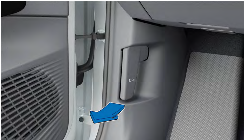
In the footwell on the driver's side: release lever for the bonnet (example ID.4).
