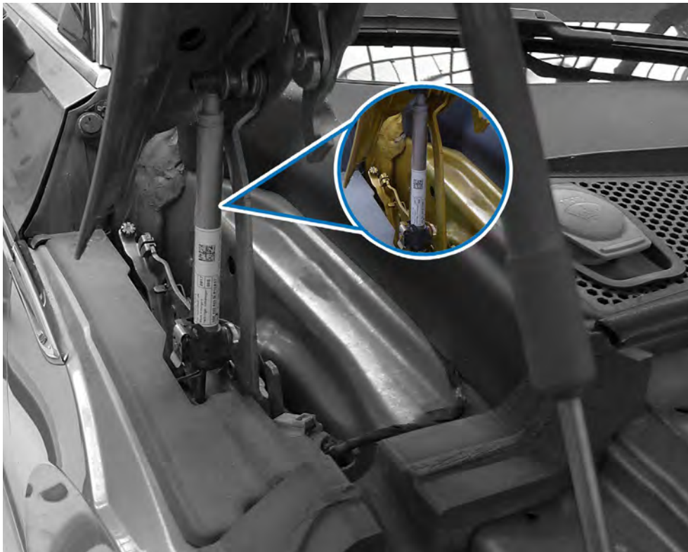
Example of a re-active bonnet with pyrotechnic actuator.
