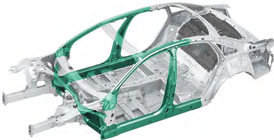
Body with reinforced passenger compartment
