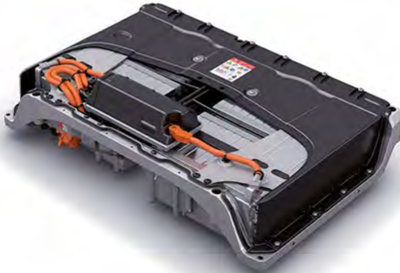
The high-voltage battery of the Passat GTE
