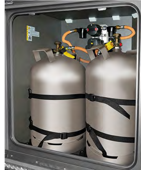
Camping gas cylinders are usually secured against slippage.
