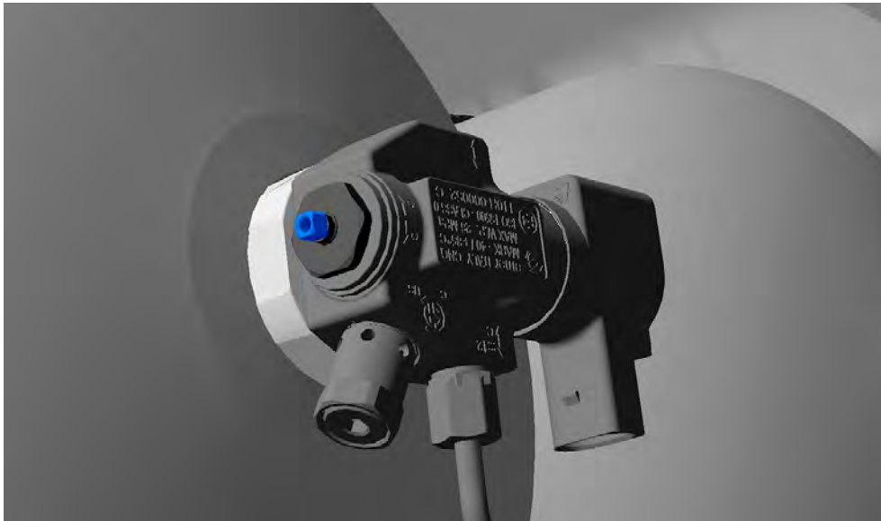
Turn the shut-off valve clockwise as far as it will go using a 5 mm open-end spanner or pliers or a special tool.
