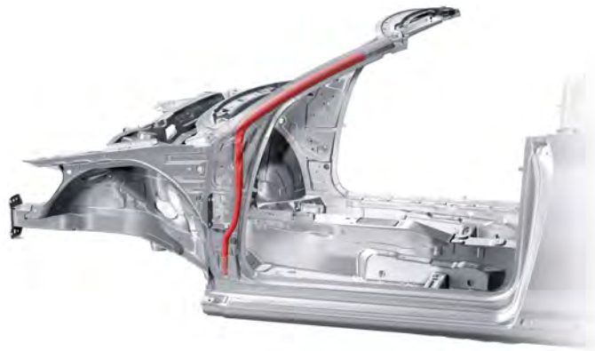
A-pillar reinforcement in cabriolets
